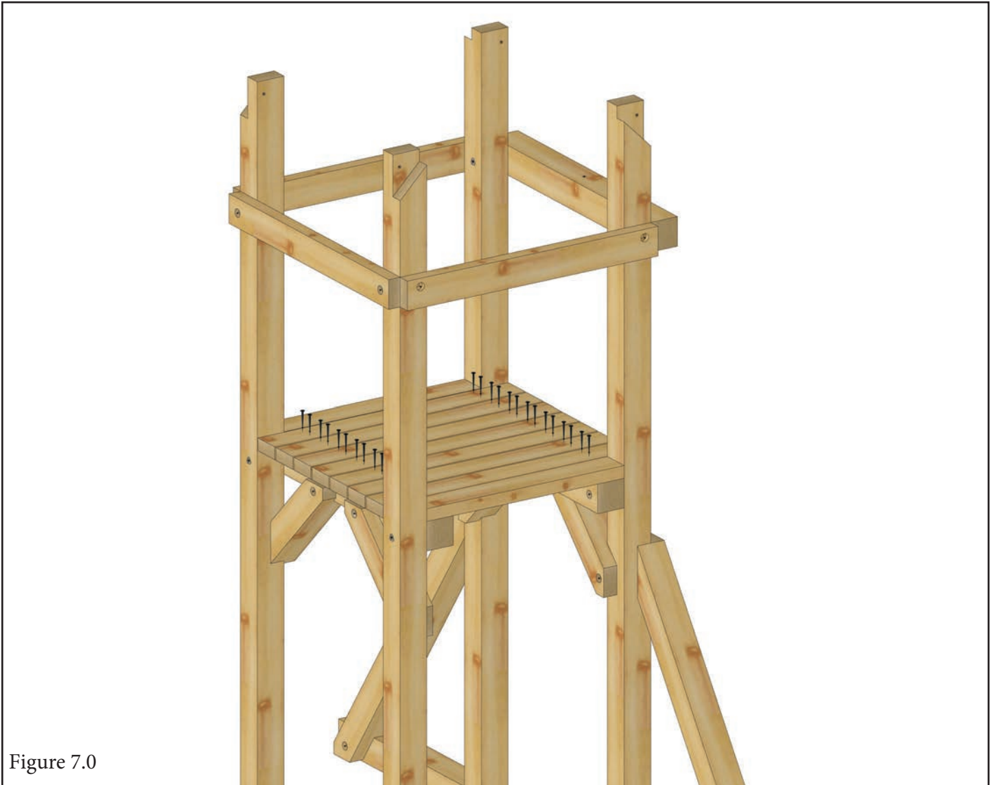
Figure 7.1 Shows how to use the screws for spreading out deck boards with even spacing.
